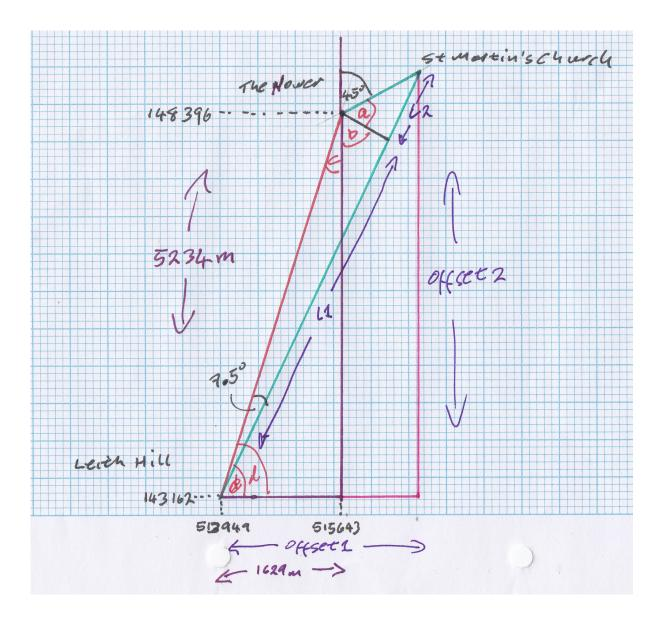
If I can find the angle e and the lengths 11 and 12 then I can use sines and cosines to find the offsets.
